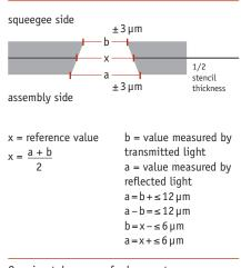
Opening tolerances of a laser cut
