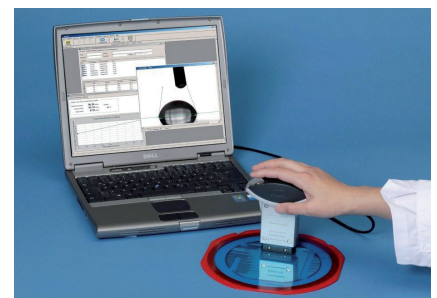
Picture 12: Computer-controlled contact angle measure equipment
