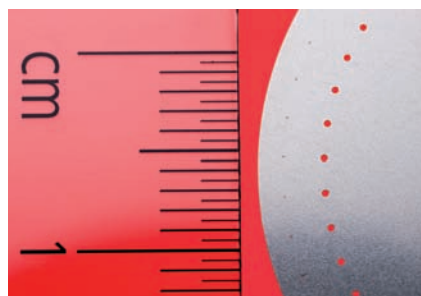
Picture 6: Measuring disc with 40 \mu\text{m} borehole
