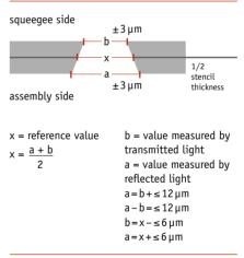
Opening tolerances of a laser cut
