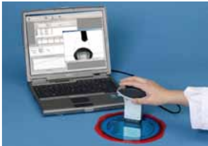
Picture 12: Computer-controlled contact angle measure equipment
